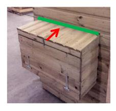
Finally knock the packing strip into place (green line) to fill the gap and using 40 mm nail fix down strip
