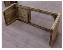
Attach both end sections of the hutch to the front section using 4x 60mm screws.
