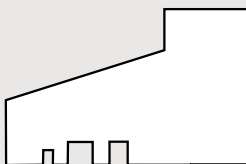
PROFILE 940 - Small Cill 70mm x 45mm
