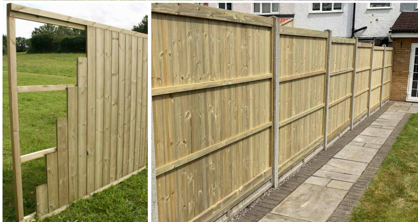
D DELUXE V JOINT TONGUE & GROOVE PANEL TGP Top & Bottom Rails 95 x 45mm | Intermediate Battens 45 x 28mm | TGV Boards 120 x 14mm Sizes: 6' x 6' 6' x 5' 6' x 4' 6' x 3'
