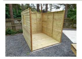
1. Place the floor section on the base you have prepared and fix the back panel to one side panel screwing through the vertical battens of the back panel into the battens on the side panel using three screws. Repeat when fitting the other side panel.
