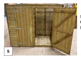
5. Take the Front Section and fix it to the  $2 \times 8$  Side Sections, using  $2 \times 60$ mm Screws on each side. Fix it to the base using  $3 \times 60$ mm Screws. (You will use  $7 \times 60$ mm Screws at this step).
